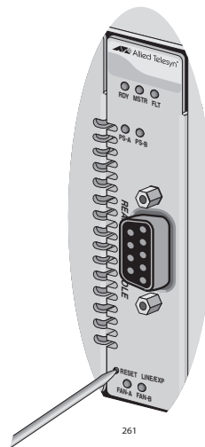
Figure 55. Resetting Converteon™ Line Cards/Rear Expansion Module
